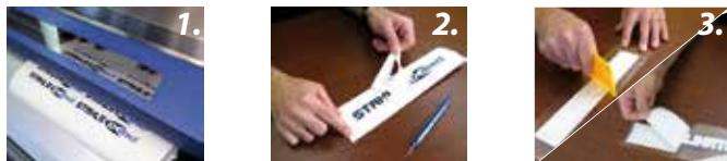
**EN** FEED MATERIAL into the printer so that the media faces up. Print design in positive form. (1)
